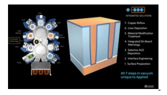
Applied Materials' new Endura® Copper Barrier Seed IMS™ combines seven different process technologies in one system under high vacuum to improve chip performance and power consumption. An animation of the process sequence can be viewed here: <a href="https://bit.ly/3g8HMe1">https://bit.ly/3g8HMe1</a>.
