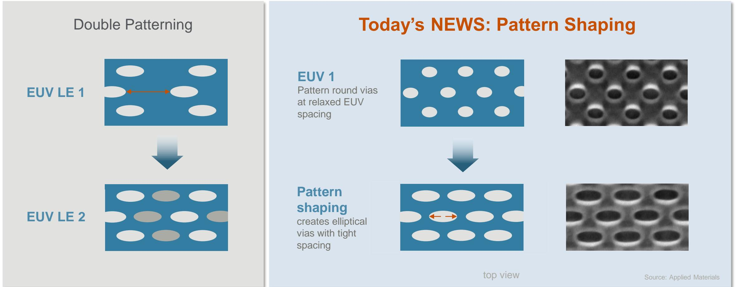
PPACt benefit: delivers high-density elliptical vias with only one EUV step, simplifying the patterning process flow – and optimizing chip power, performance, area and cost
