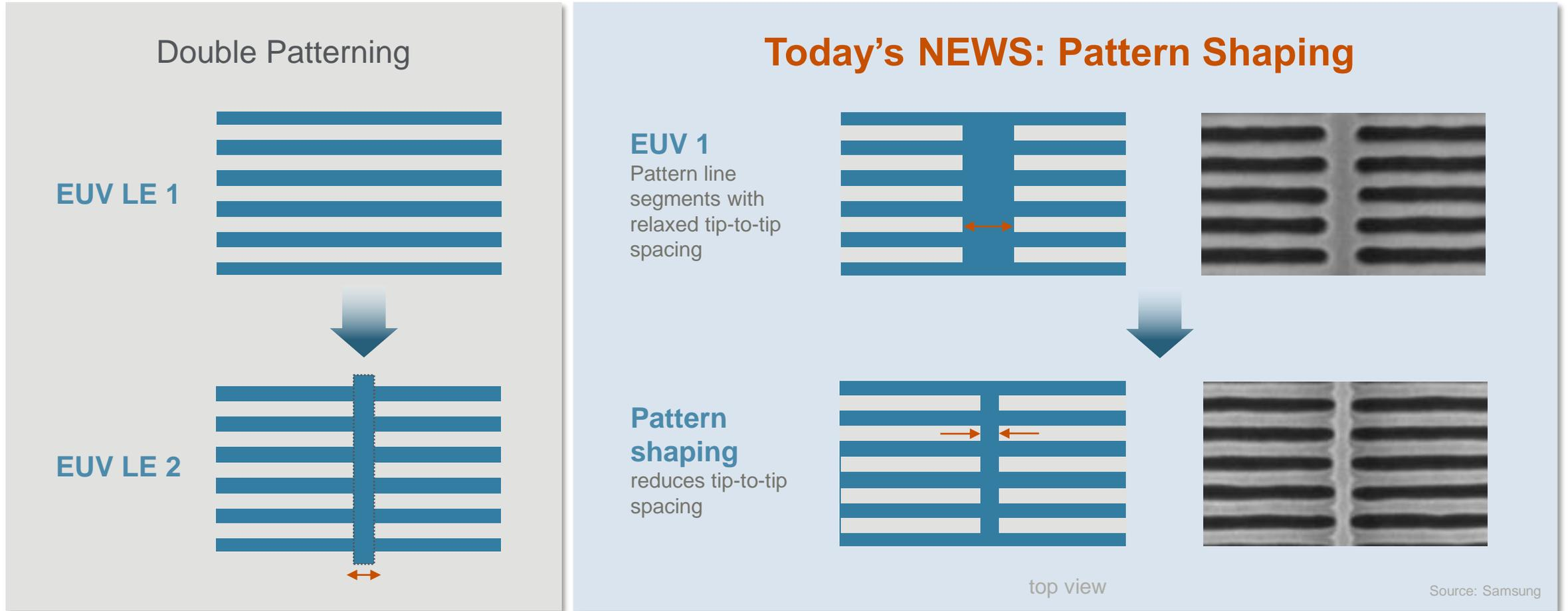
PPACt benefit: delivers the density of EUV double patterning with only one EUV step, simplifying the patterning process flow and optimizing chip area and cost
