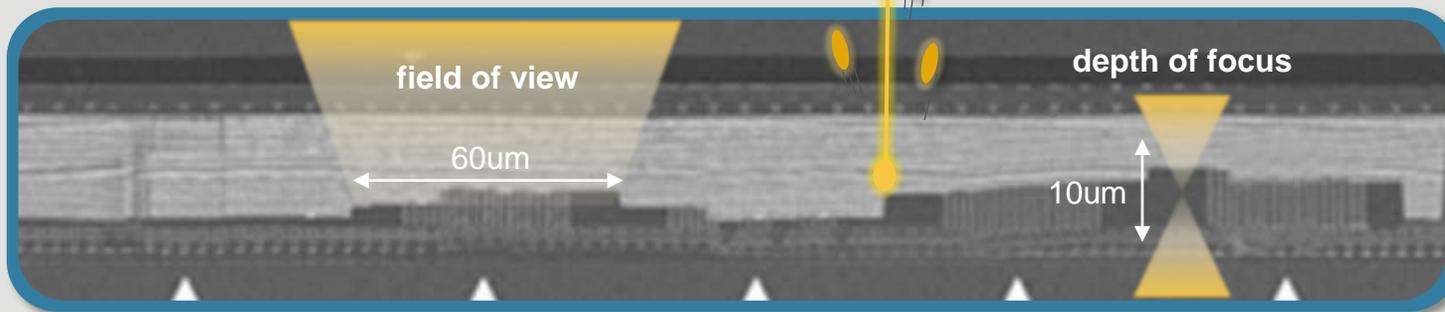
**Staircase interconnect architectures** increase contact density to reduce die area and cost. VeritySEM® 10 uses a large field of view with high depth of focus to measure the entire staircase structure with detailed step widths that help tune etch process recipes.
