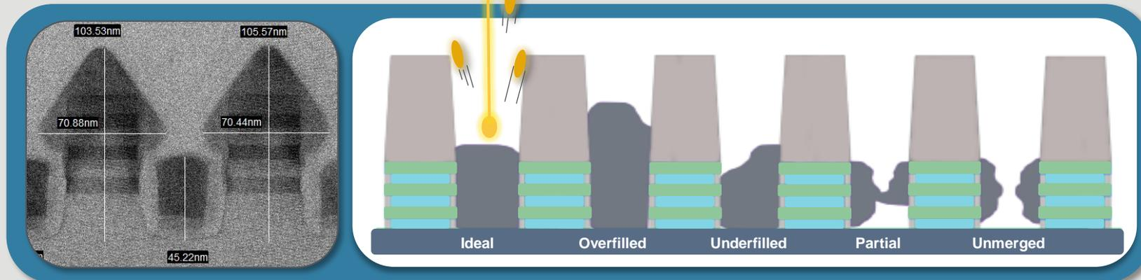
**Selective epitaxy** is key to GAA nanosheet engineering. VeritySEM® 10 uses BSE technology to measure and characterize the epitaxy process.
