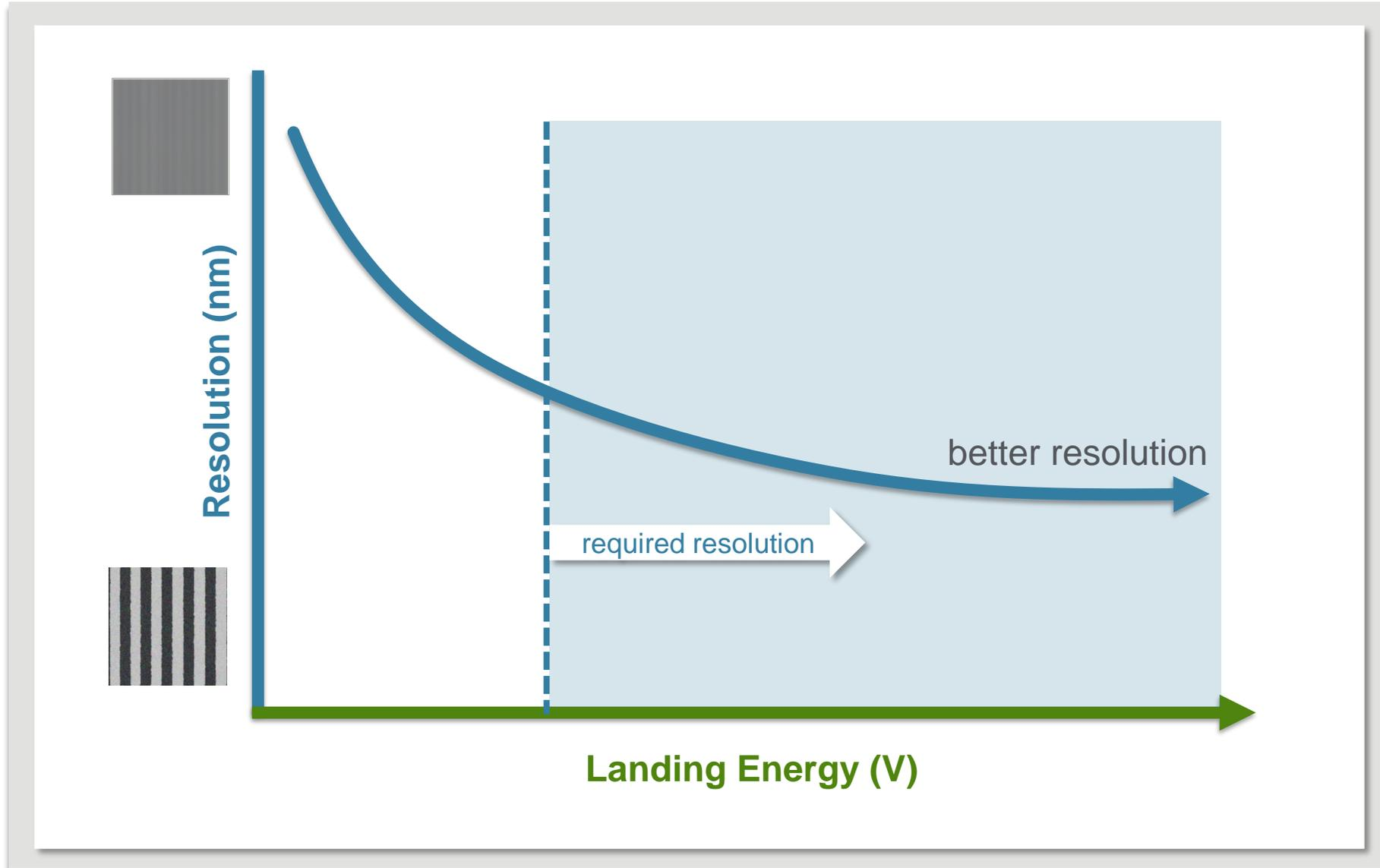
**Landing energy:** high energy is used to concentrate the electron beam on the target area and produce higher resolution images.
