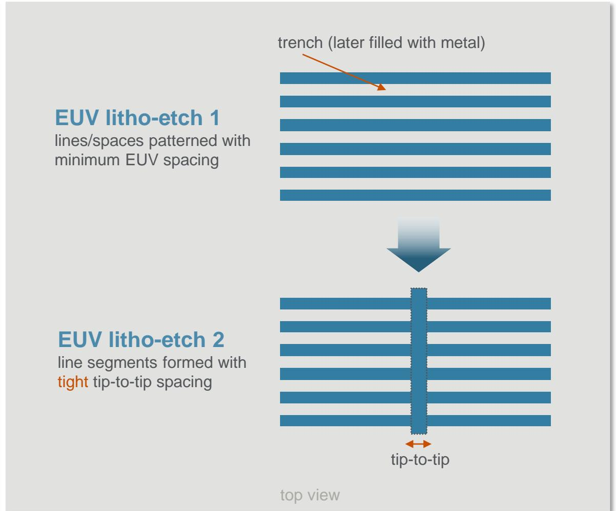
Tighter tip-to-tip spacing enables higher device density, which optimizes die area
